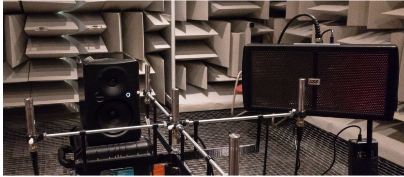
Figure 5.2: Experimental setup. The five-microphone orthogonal probe has a radius of a = 0.25 m. The loudspeaker was used as the source for both experiments, while the parametric speaker array was used as the noise source for the phase gradient adjustment experiment.
