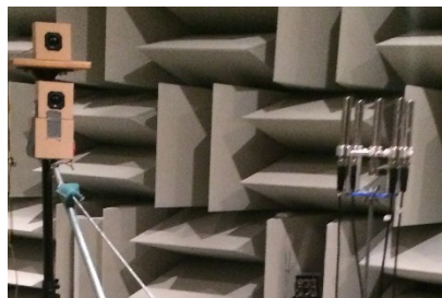
Figure 3.7: Experimental setup. The source loudspeaker location is fixed, while the additive noise loudspeaker is on a rotating arm to have variable angular separation.
